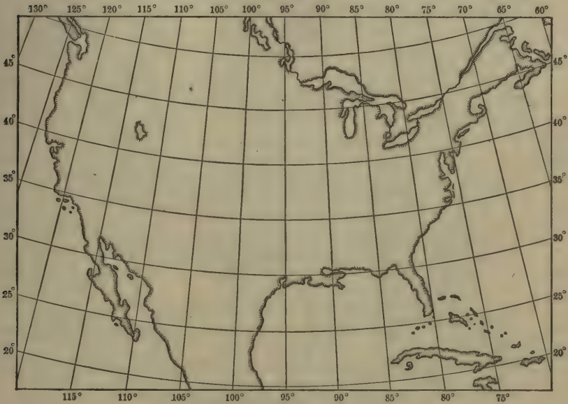
FIG. 100. Simple Conic Projection.
